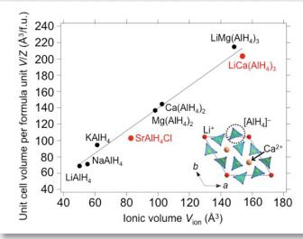
Figure 1 Crystal structure map of  $M(AlH_4)_n$ . The inset is the crystal structure of LiCa(AlH<sub>4</sub>)<sub>3</sub> [4]. Red indicates discoveries in this project.
